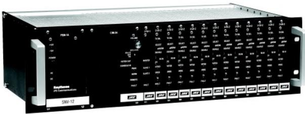
*The unit shown has a full complement of 12 SVM-2 Site Voter Modules. As many as three chassis can be daisy-chained together, allowing a voted channel with up to 36 voting receiver sites!*
