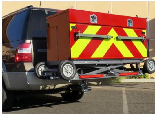
**Accessories** - Each unit is outfitted with a firearms lock-box, full size filing cabinet, laptop charging drawer, shelves and drawers for organization, slide out platform for the printer/scanner, scene lights, (2) T-Card arms, white board and drop down stabilization legs.
