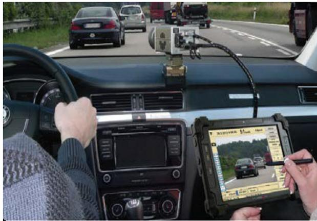
PM-511 can support radar and camera for the purpose of speed violation detection. Once the tablet is connected on the detection devices, the captured vehicle information such as car model, license plate, car speed, driver information and other details will be displayed on the tablet and sent to headquarters for analysis. This information allows the officer to quickly determine the related fines, without wasting time on redundant paperwork.
