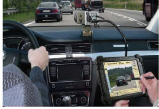
PM-511 can support radar and camera for the purpose of speed violation detection. Once the tablet is connected on the detection devices, the captured vehicle information such as car model, license plate, car speed, driver information and other details will be displayed on the tablet and sent to headquarters for analysis. This information allows the officer to quickly determine the related fines, without wasting time on redundant paperwork.
